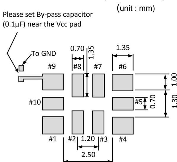
To maintain stable operation, provide a 0.1μF by-pass capacitor at a location as near as possible to the power source terminal of the crystal product (between Vcc - GND).
