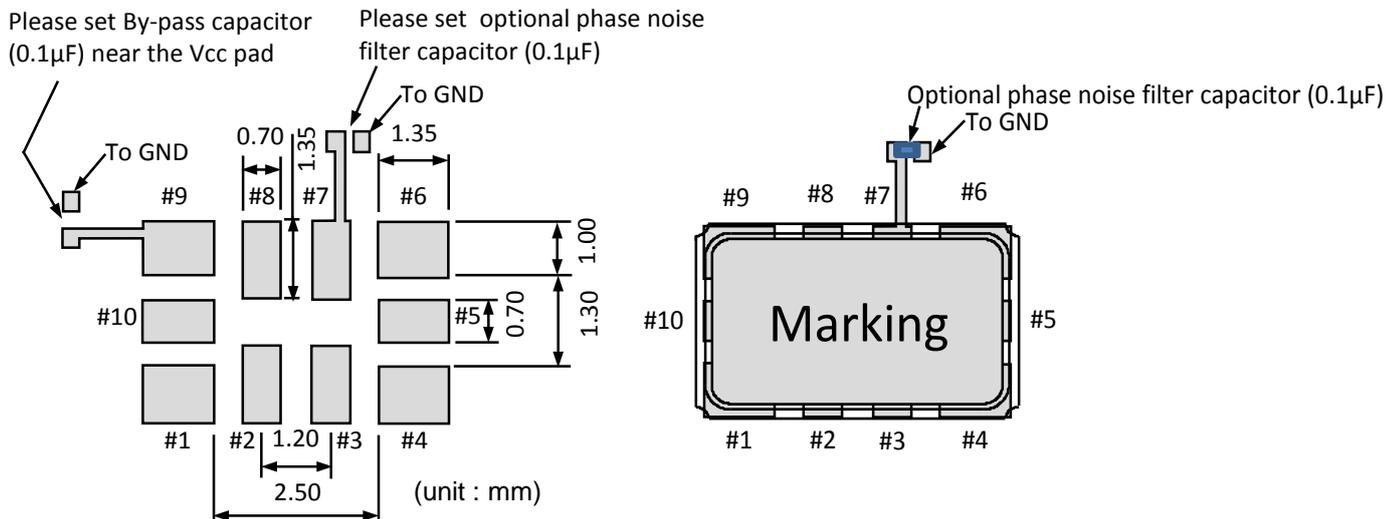
To maintain stable operation, provide a 0.1μF by-pass capacitor at a location as near as possible to the power source terminal of the crystal product (between Vcc - GND).
