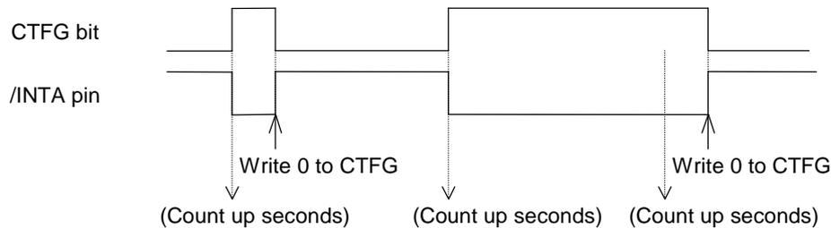
Note: When using the clock precision adjustment function, the periodic interrupt's cycle changes once every 20 seconds.
