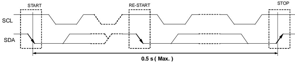
1) START condition, repeated START condition, and STOP condition
