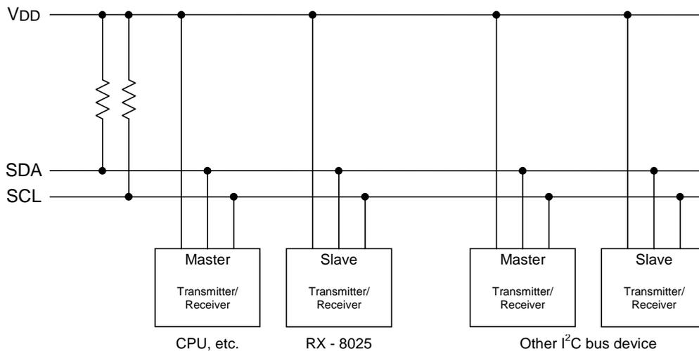
Any device that controls the transmission and reception of data is defined as a master device and any device that is controlled by a master device is defined as a slave device.
