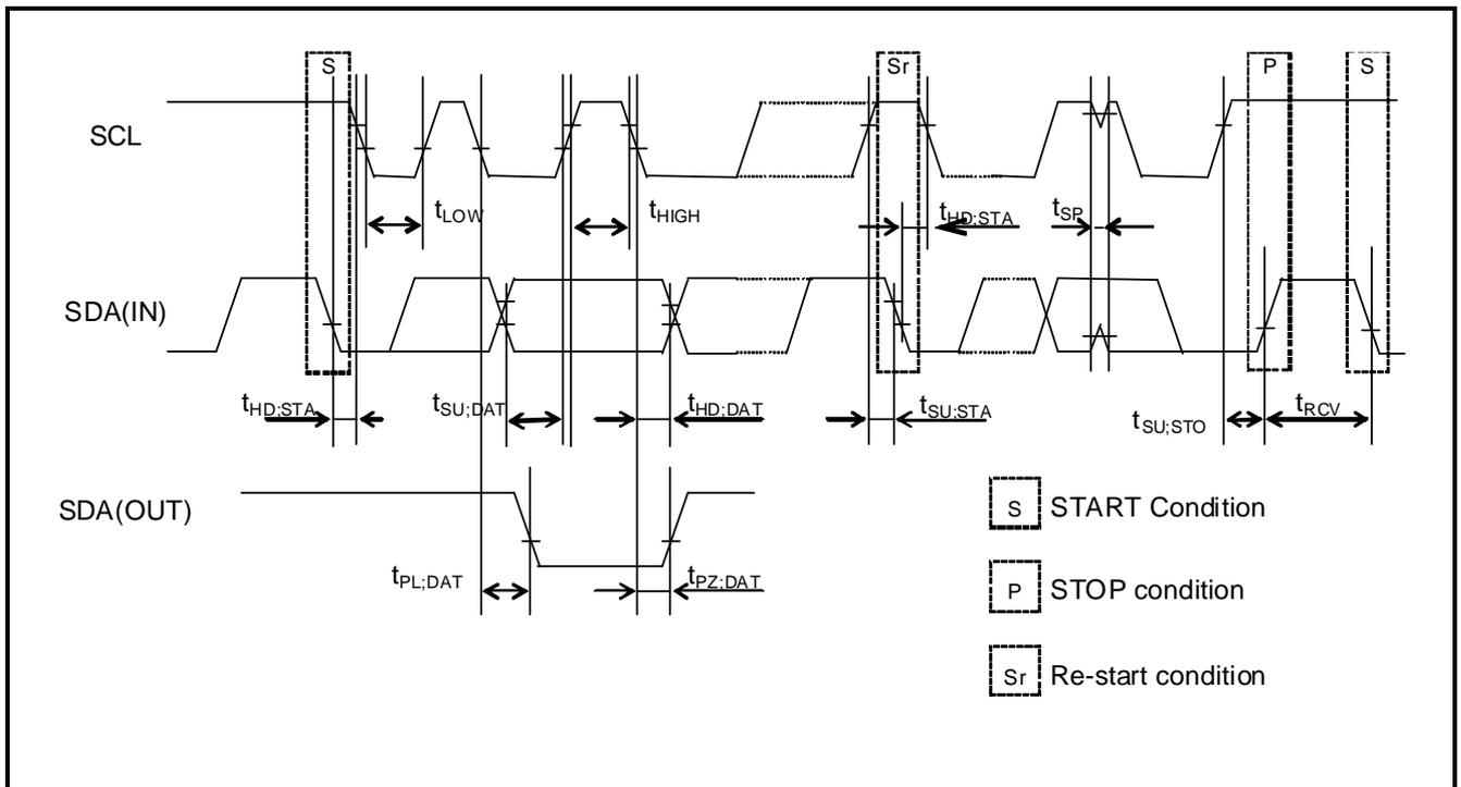
Caution: When accessing this device, all communication from transmitting the start condition to transmitting the stop condition after access should be completed within 0.5 seconds. If such communication requires 0.5 to 1.0 second or longer, the I<sup>2</sup>C bus interface is reset by the internal bus timeout function. Please see also 8.8.3. Starting and stopping I<sup>2</sup>C bus communications.
