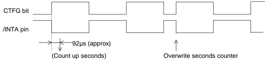
Note 1: As is shown in the above diagram, the seconds register's count up operation occurs approximately 92 µs after the falling edge of the /INTA output. Therefore, if the clock's value is read immediately after the output's falling edge, the read clock value may appear to be about one second slower than the RTC module's clock value.
