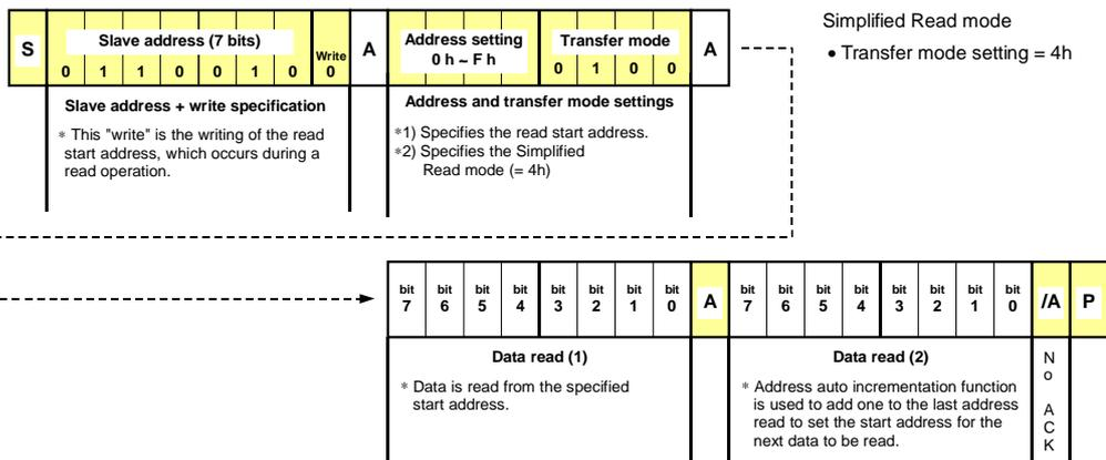
(3) Read method from address Fh, with no specified start address for read operation
