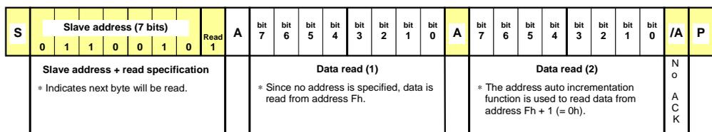
\* The above steps are an example of transfers of one or two bytes only. There is no limit to the number of bytes transferred during actual communications. (However, the transfer time must be no longer than 0.5 seconds and access to the Address Dh (Reserved) register is prohibited.)
